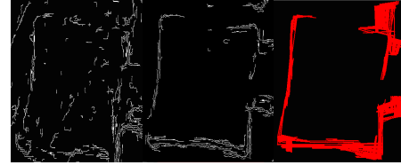
Fig. 6. Workflow of processing image within bounding box. Image on the left shows the initial Canny edge detection result and the middle image shows the final Canny edge detection result after dynamically chosen gaussian kernel size and the image on the right shows the hough filter result, which is used in the following GVF snake.
