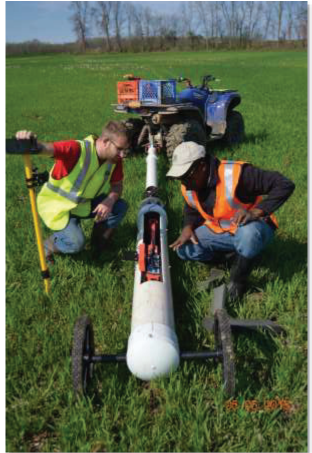
Figure 1: The EM38-MK2 instrument mounted in a custom-made cart for the electromagnetic induction survey.
